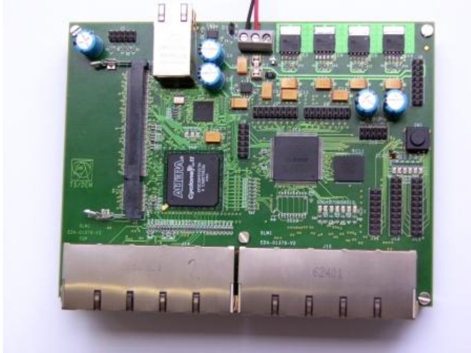
Figure 39: The SLM (Smart Link Module) board.
