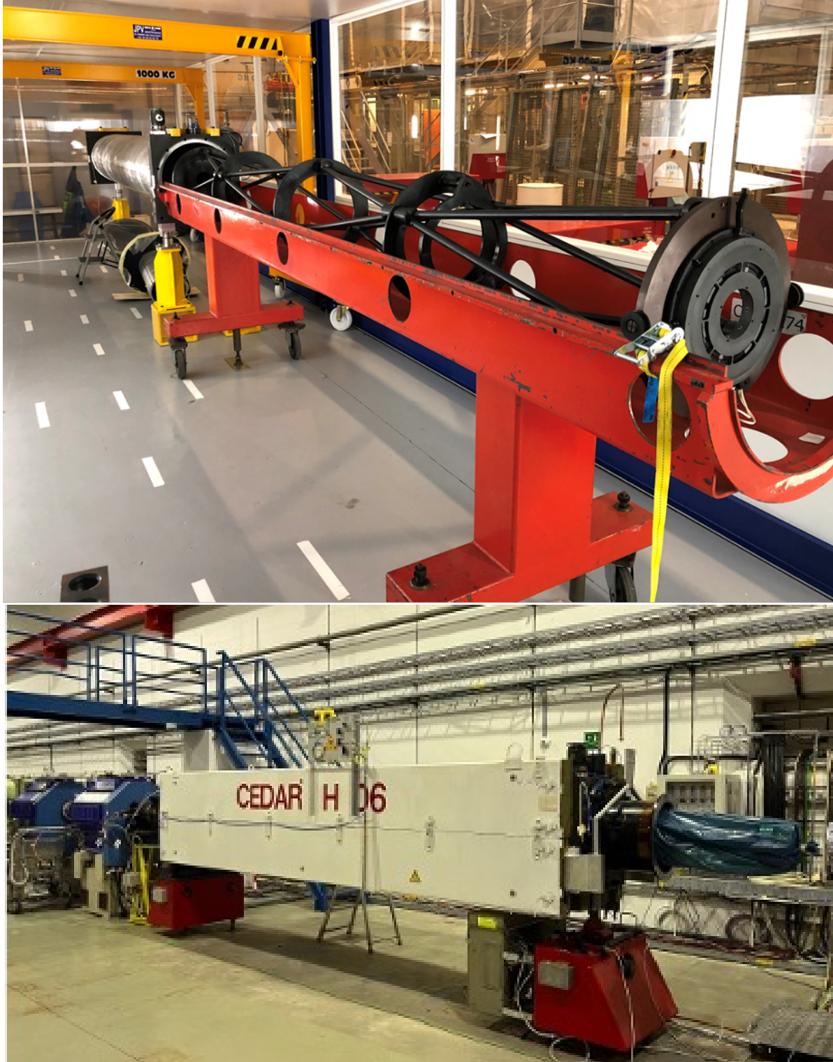
Figure 3: Top: The CEDAR detector is positioned in a Grey room at CERN; then the internal optics is extracted from the vessel to be replaced with new components. Bottom: The CEDAR with optics optimised for H_2 is installed on the NA62 beam line; the KTAG detector (hosting photon collection and detection systems) is then mounted on the upstream end. The blue plastic surrounding the CEDAR nose protected the quartz windows during transportation.
