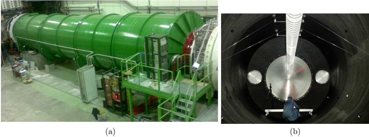
Figure 26: (a) The RICH vessel installed in the NA62 cavern. (b) The beam pipe seen from inside the RICH vessel; the entrance window and the location of the PMTs disks can clearly be seen
