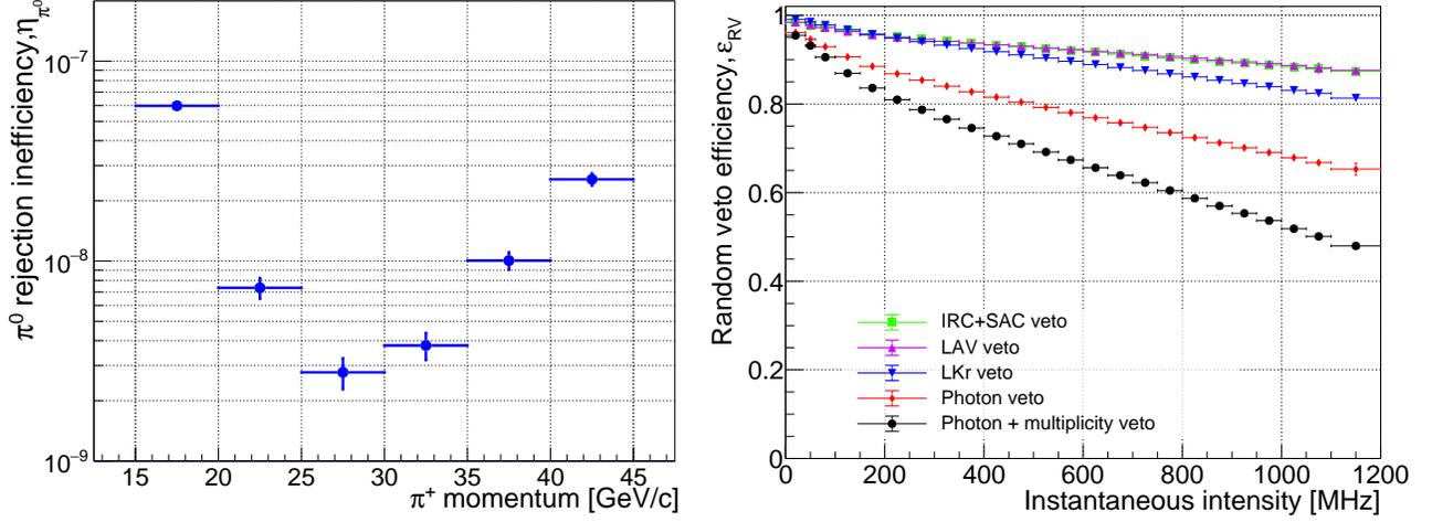
Figure 3: Left:  $\pi^0$  rejection inefficiency (defined as in figure 3-left of [3]) as a function of the  $\pi^+$  momentum in 2024 data. Right: random veto efficiency (defined as in figure 4-right of [3]) as a function of the instantaneous beam intensity in 2024 data.
