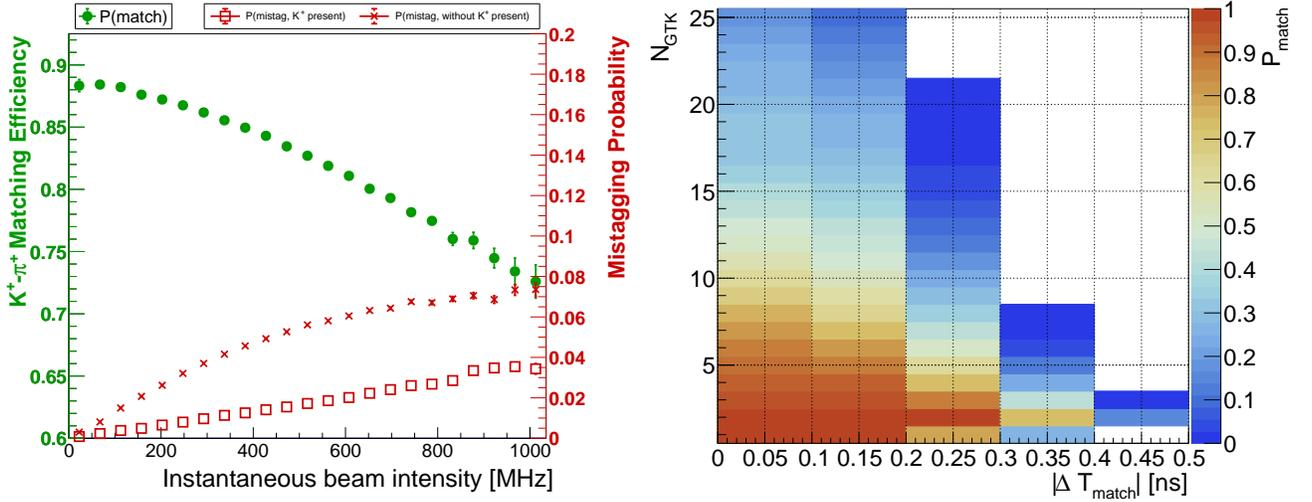
Figure 4: Left:  $K^+-\pi^+$  matching performance, showing the efficiency of the matching (green, left vertical axis) and the probability of ‘mistagging’ an incorrect GTK candidate as the parent  $K^+$  of a selected  $\pi^+$  (red, right vertical axis), measured in a  $K^+ \rightarrow \pi^+\pi^+\pi^-$  control sample in 2024 data. Right: matching probability (defined as in figure 9-right of [3]) measured in the  $K^+ \rightarrow \pi^+\pi^0$  normalization sample in 2024 data.
