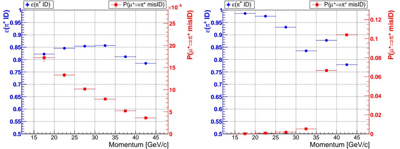
Figure 2: Particle identification performance (defined as in figure 2 of [3]) as a function of momentum, using information from LKr, MUV1,2 and MUV3 (left), and from RICH (right), in 2024 data. The  $\pi^+$  identification efficiency is shown as blue circles (left vertical axis) and the probability of mis-identification of a  $\mu^+$  as a  $\pi^+$  is shown as red squares (right vertical axis).
