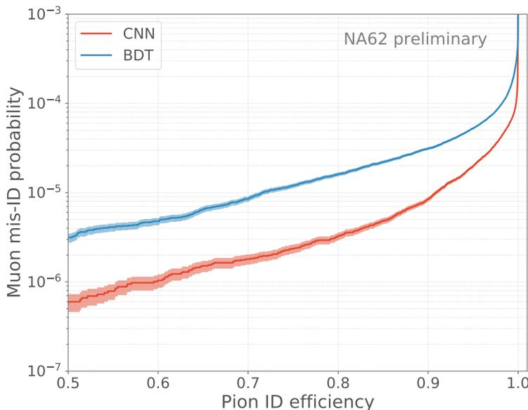
Figure 5: Calorimeter muon mis-ID probability as a function of the pion ID efficiency for events with momentum in the 15 to 50 GeV/c range. The newly developed CNN method is shown in red and the existing BDT based approach is indicated in blue. Those curves were obtained with the 2018 data set.
