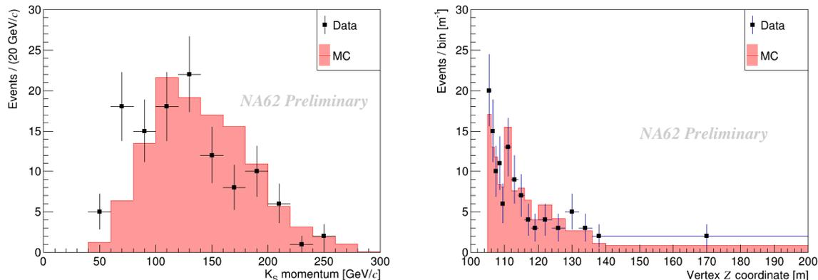
Figure 8: Distributions from reconstructed  $K_S \rightarrow \pi^+\pi^-$  decays: momentum (left) and  $Z$ -coordinate of the decay vertex (right). Data corresponding to  $1.6 \times 10^{16}$  POT (117 events, black dots, error bars statistical only) are compared to simulation data obtained from a combination of the G4BeamLine and NA62MC Monte Carlo software (red, normalized to the data integral).
