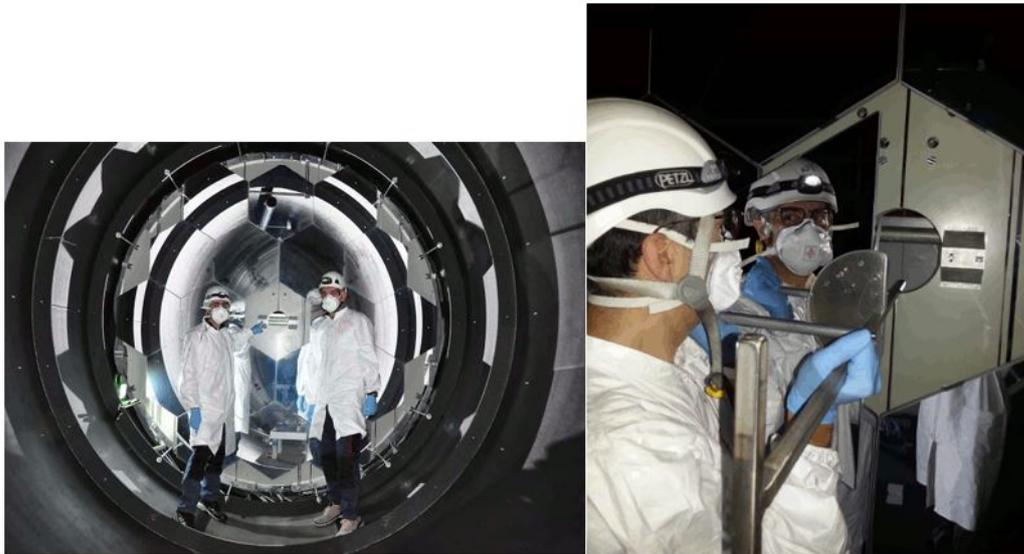
Figure 21: Left: Front view of the mirror system after the two central semi-hexagonal mirrors have been removed. Right: Installation of one of the two new semi-hexagonal mirrors.
