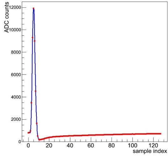
Figure 19: A calibration pulse, taken with 128 samples
