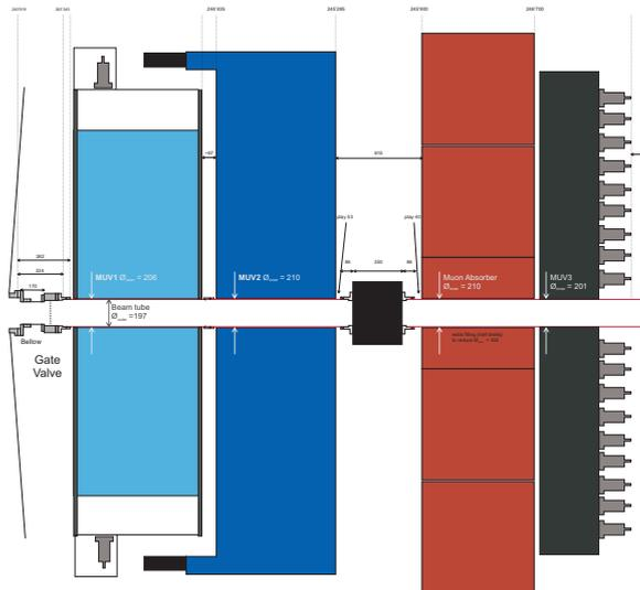
Figure 20: General set-up of the three muon veto detectors MUV1, MUV2, and MUV3
