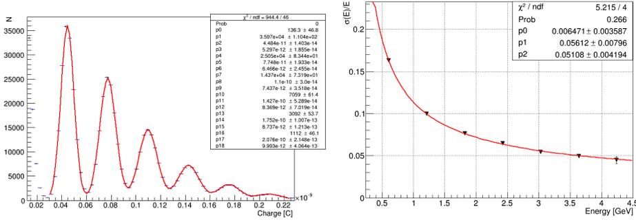
Figure 15: Charge measured by the SAC at the BTF test run (left) together with the obtained energy resolution (right)
