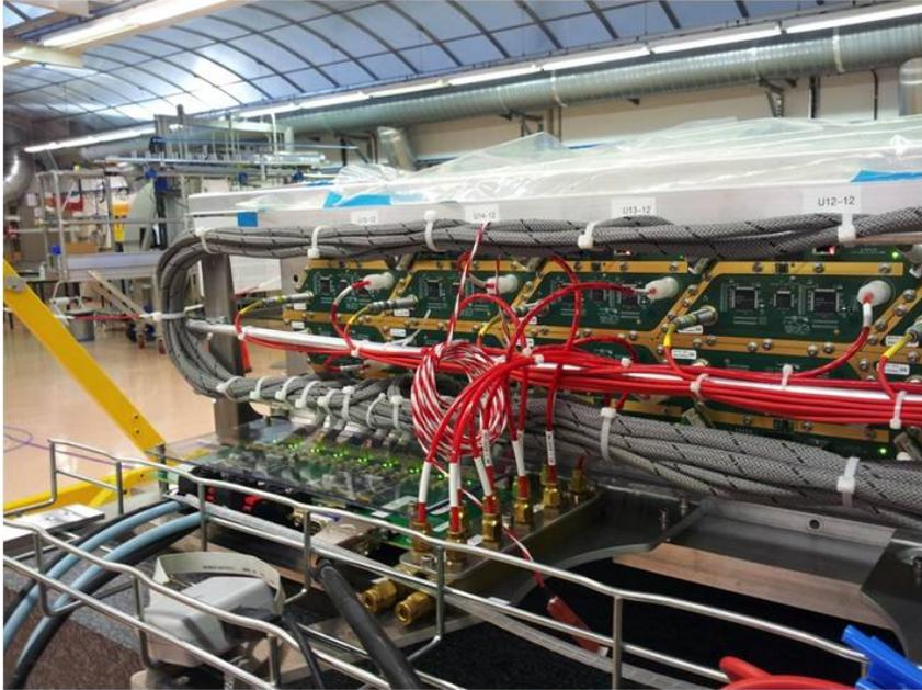
Figure 13: The dressing of a Straw module
