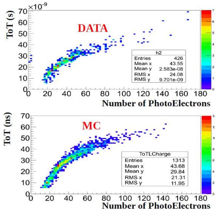
Figure 12: A DATA-MC comparison for the detailed simulation of a CHANTI bar. The simulation refers to a MIP, the data is from a cosmic ray tests, the threshold chosen is 80 mV.
