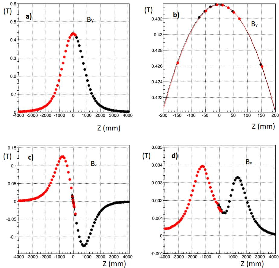
Figure 2: Examples from the B-field measurements: a)  $B_y$  (X=28 cm, Y=44 cm) versus Z; b) same as a) with zoomed scales; c)  $B_z$  (X=28 cm, Y=44 cm) versus Z; d)  $B_x$  (X=28 cm, Y=44 cm) versus Z. Note: Z=0 is in the centre of the magnet
