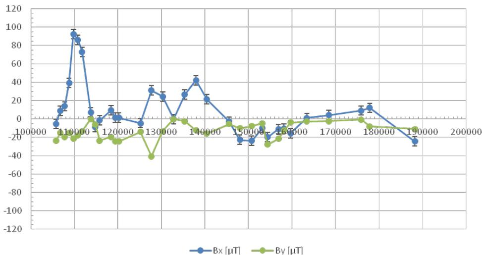
Figure 3: Residual B-fields in  $B_x$  and  $B_y$  in the vacuum tank over a length of 85 m. The horizontal axis is the Z axis of the experiment in mm, starting shortly after GTK3 and ending after the MNP33 magnet. The MNP33 magnet was off during these measurements
