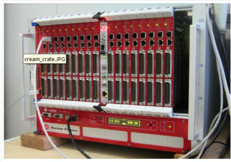
Figure 16: Pre-series of the CREAM modules delivered by CAEN
