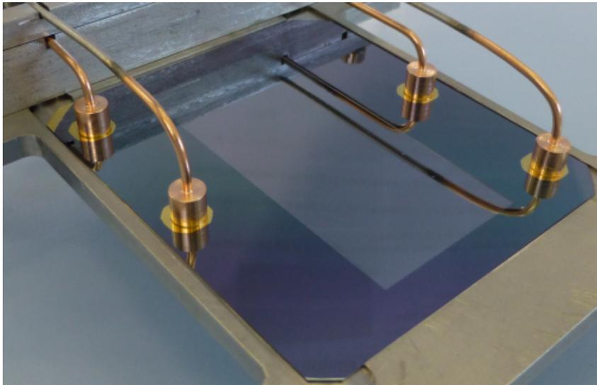
Figure 9: Miniaturized soldered Kovar connectors
