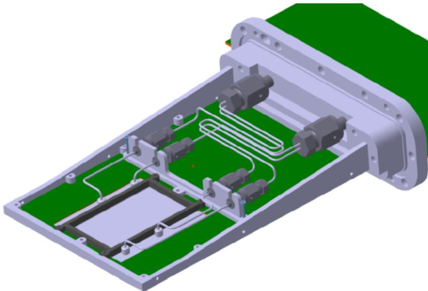
Figure 10: Integration of the "cold module" onto the GTK PCB, including the tubing and the sealing flange
