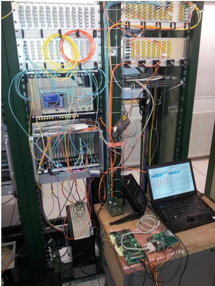
Figure 22: The GTK test readout setup during the November 2013 dry run
