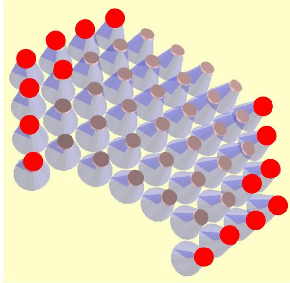
Figure 6: The PMT hybrid matrix. The position of the 16 R7400 PMTs are highlighted in red
