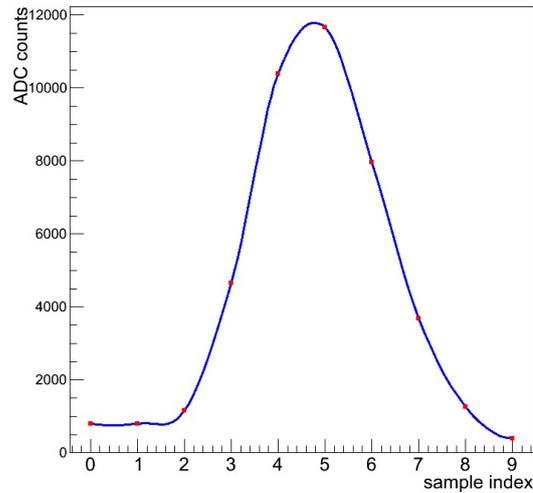
Figure 18: A typical calibration pulse, taken with 10 samples
