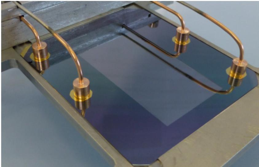
Figure 9: Miniaturized soldered Kovar connectors
