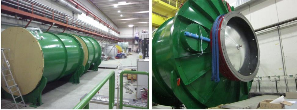
Figure 14: Left: two RICH vessel sections in the NA62 cavern. Right: the first section of the RICH vessel, with the conical cap and the entrance window already installed
