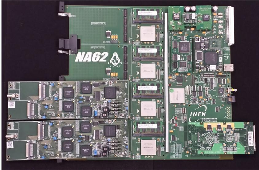
Figure 21: The V3 TEL62 board with larger FPGAs and power-distribution daughter-card and two TDCB plugged in
