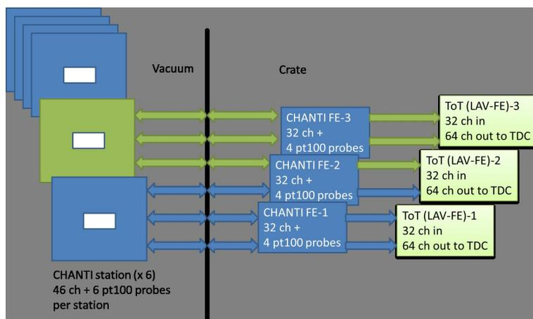
Figure 11: A schematic view of CHANTI two level FEE.
