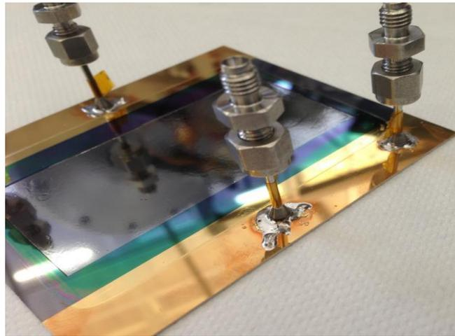
Figure 8: One device from the IceMOS production, post-processed by PH-DT, prior to installation in the test vessel for thermo-hydraulic characterisation
