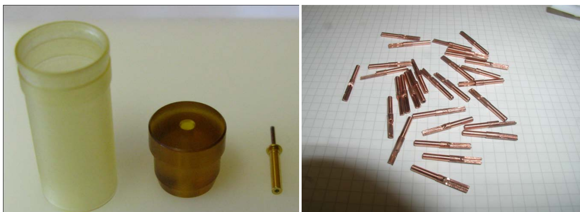
Figure 36. Details of the straw end-pieces are shown. The socket is glued between the straw and the structure (left). The connection plug pushes the petals of the web to the straw wall. The crimp-tubes connect the wire to the Kapton® layer of the web circuit by crimping (left picture) or by soldering (right picture).
