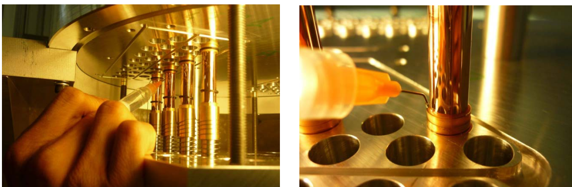
Figure 52. Bottom side gluing (left) and the gluing of the top side (right).
