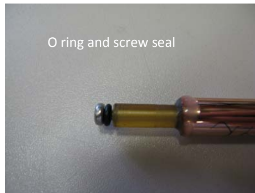
Figure 26: The PEI non-return valve (left) and the opposite side with O ring and an M4 screw.
