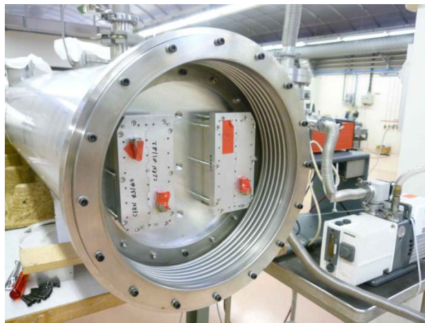
Figure 60. View of the far end with the metallic bellows for the vacuum and leak test. The two gas cells (without electronics) are visible in the center.
