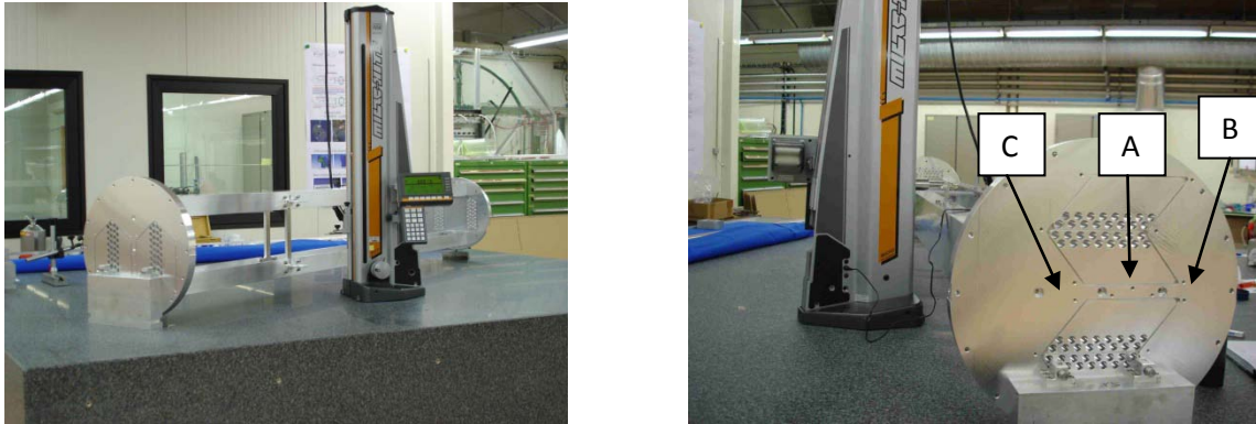
Figure 49. View of the prototype structure (left) and the measurement of the frame on the granite table.
