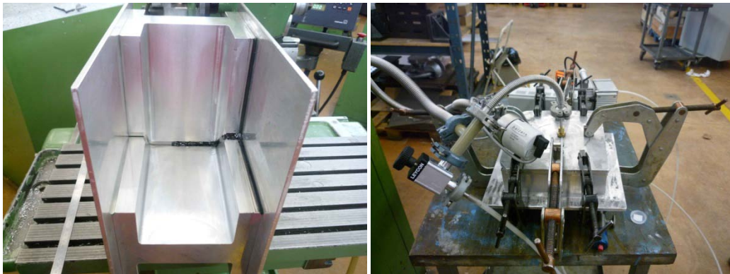
Figure 34. Prototype detector's inner corner (left) and a set-up verify leak tightness (right).
