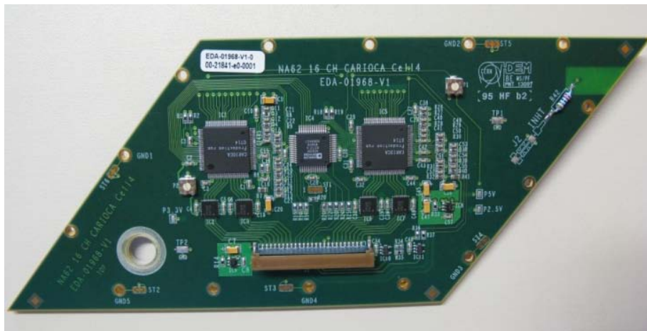
Figure 38. Front-End board (cover) with the two CARIOCA chips (front side). The cover is mounted on partition serves as a leak-tight roof for the gas manifold and fed through for gas, high-voltage and signal connections to the straws (back side).
