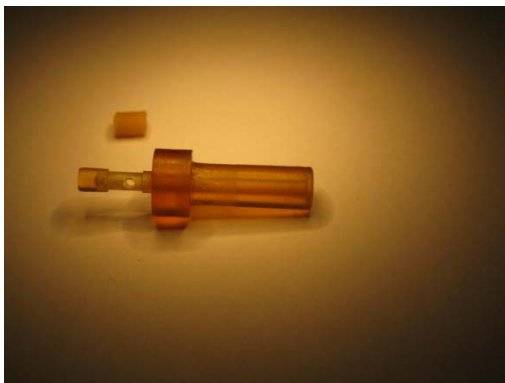
Figure 26: The PEI non-return valve (left) and the opposite side with O ring and an M4 screw.
