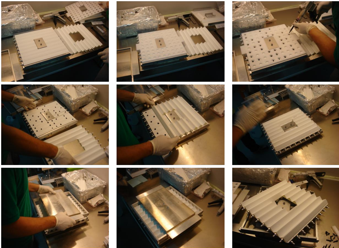
Figure 139 Assembling "First step": a) A half-layers is arranged on the jig, b) Teflon mask is aligned, c) Glue spots are applied, d) Mask is removed, e) f) Bars of the other half-layer are placed, g) h) second jig is applied on top to align last placed half-layer and to redistribute pressure, i) Half-module as appear the day after gluing
