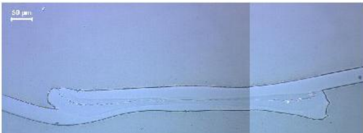
Figure 240. Cross section of a welded seam where the two sides of the strips are fused.
