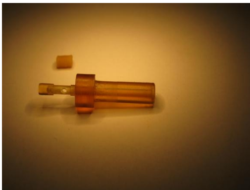
Figure 245: The PEI non-return valve (left) and the opposite side with O ring and an M4 screw.
