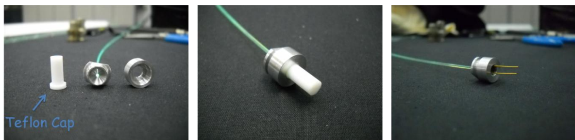
Figure 133 a) Connector in its parts b) Assembled connector c) Connector with SiPM
