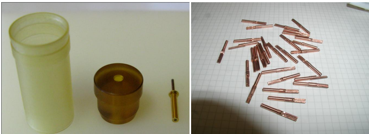
Figure 255. Details of the straw end-pieces are shown. The socket is glued between the straw and the structure (left). The connection plug pushes the petals of the web to the straw wall. The crimp-tubes connect the wire to the Kapton® layer of the web circuit by crimping (left picture) or by soldering (right picture).
