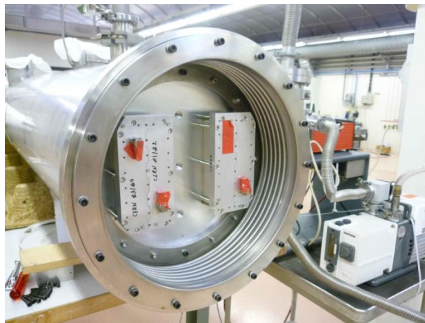
Figure 279. View of the far end with the metallic bellows for the vacuum and leak test. The two gas cells (without electronics) are visible in the center.
