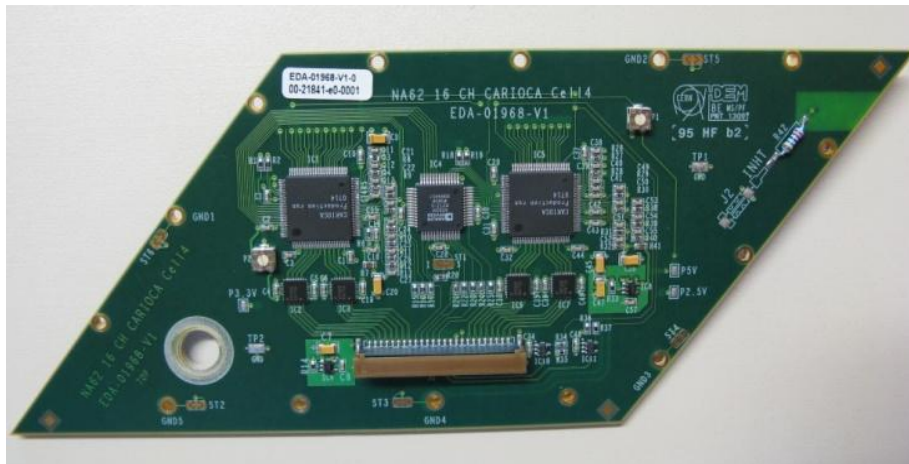
Figure 257. Front-End board (cover) with the two CARIOCA chips (front side). The cover is mounted on partition serves as a leak-tight roof for the gas manifold and fed through for gas, high-voltage and signal connections to the straws (back side).
