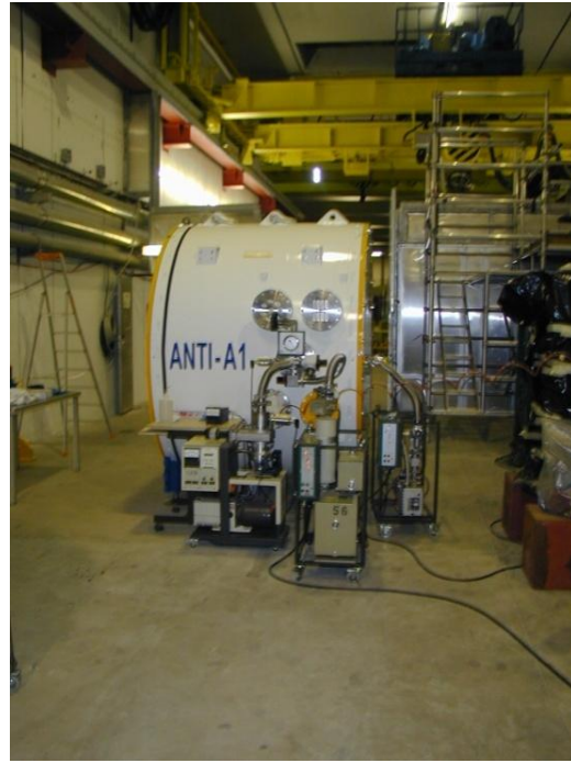
Figure 197 Vacuum test before the installation
