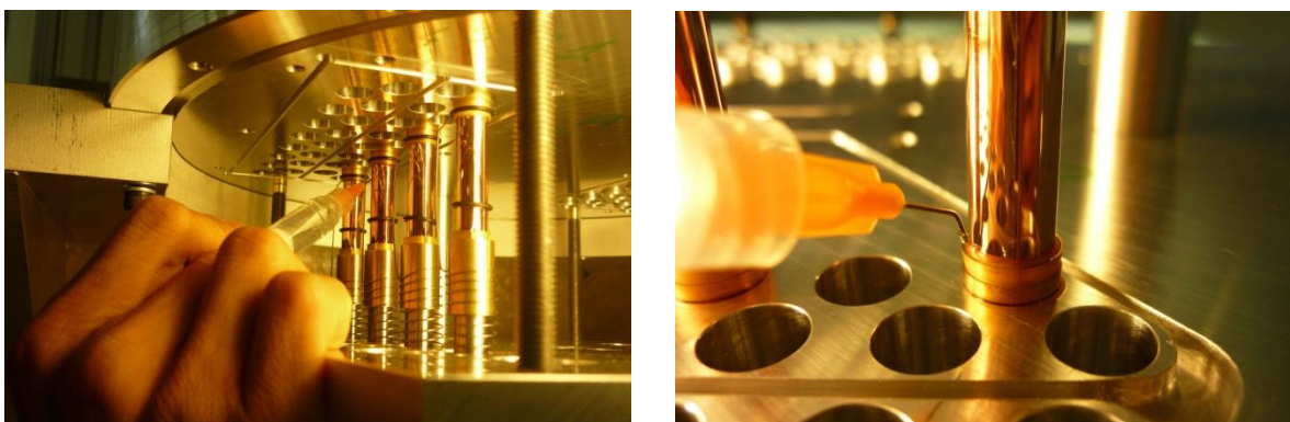
Figure 271. Bottom side gluing (left) and the gluing of the top side (right).
