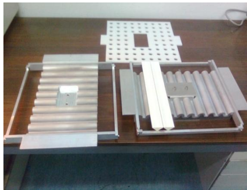
Figure 138 Jig used to align bars during gluing, on top Teflon mask to distribute glue spot
