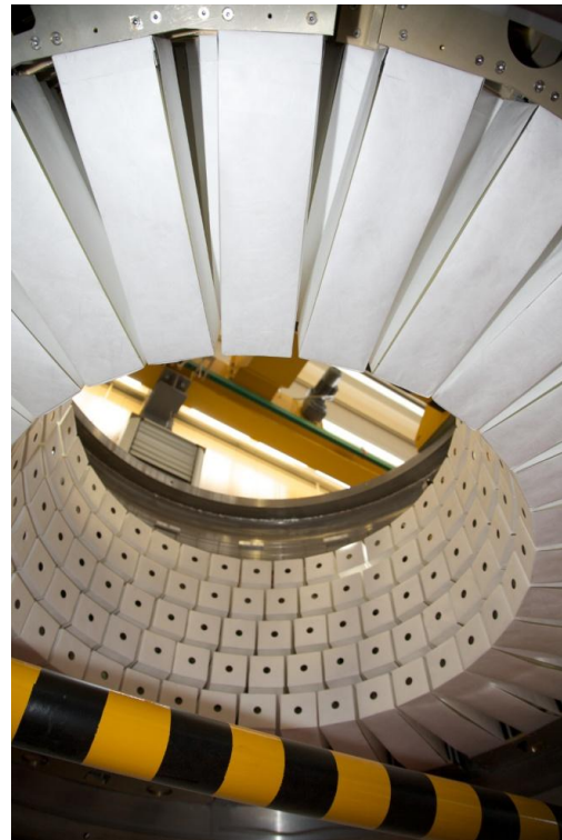
Figure 192 Inside view of one completed LAV module.
