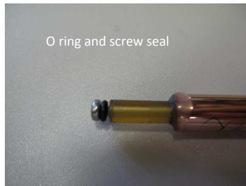
Figure 245: The PEI non-return valve (left) and the opposite side with O ring and an M4 screw.
