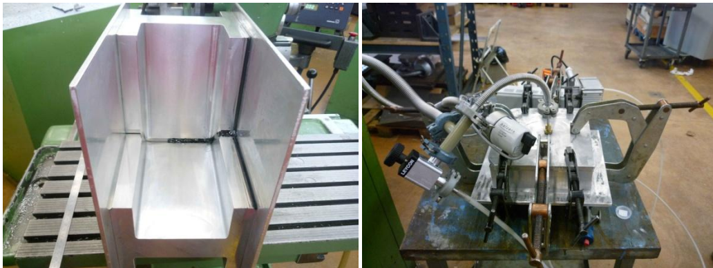
Figure 253. Prototype detector's inner corner (left) and a set-up verify leak tightness (right).
