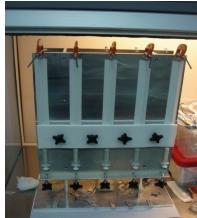
Figure 135 The fiber-bar gluing tool in action. Its back side is identical to the one shown. Glue is injected from bottom using syringer.
