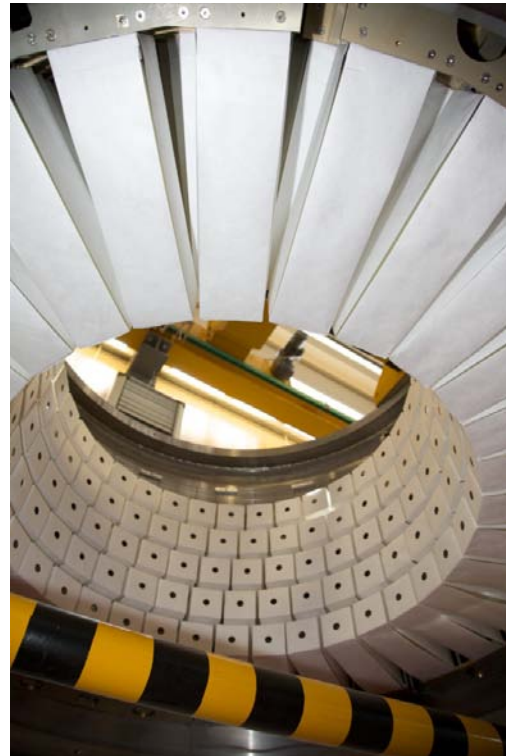
Figure 44 Inside view of one completed LAV module.
