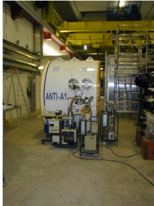
Figure 49 Vacuum test before the installation
