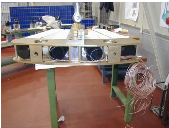
Figure 38 A complete azimuth segment with four crystals.
