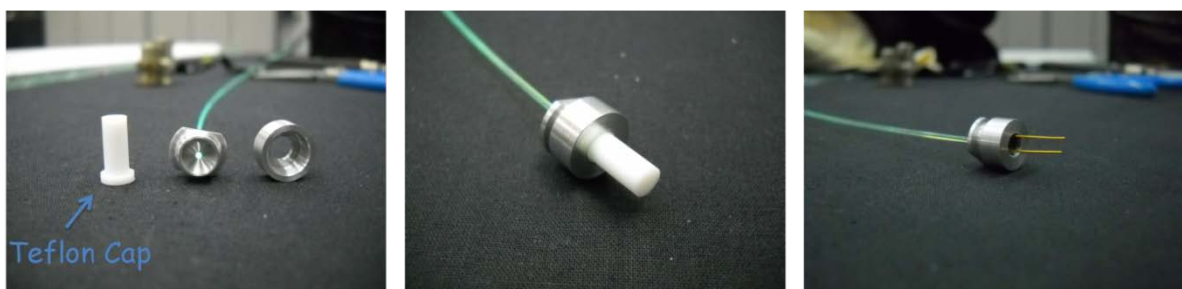
Figure 11 a) Connector in its parts b) Assembled connector c) Connector with SiPM
