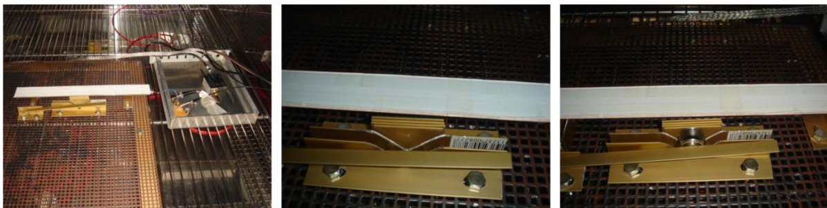
Figure 14 Experimental apparatus for bar test. a) Setup overview on the right the readout electronics and amplifier. b) Collimator detail. c) Source in final position.
