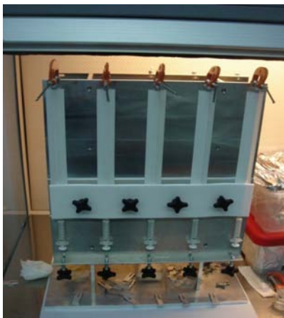
Figure 13 The fiber-bar gluing tool in action. Its back side is identical to the one shown. Glue is injected from bottom using syringer.
