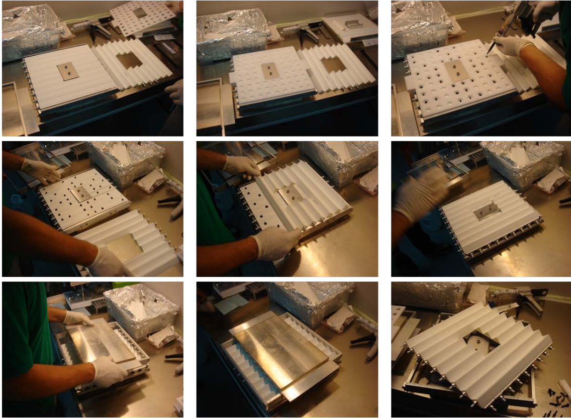
Figure 17 Assembling "First step": a) A half-layer is arranged on the jig, b) Teflon mask is aligned, c) Glue spots are applied, d) Mask is removed, e) f) Bars of the other half-layer are placed, g) h) second jig is applied on top to align last placed half-layer and to redistribute pressure, i) Half-module as appear the day after gluing
