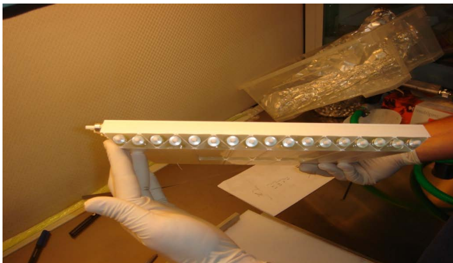
Figure 4 Staggering of triangular scintillator bars to form a plane
