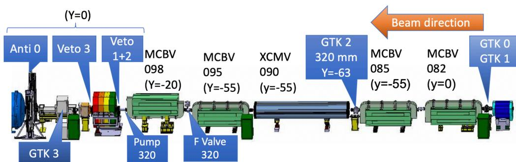
Figure 2: Schematic layout of the new achromat and beam line.
