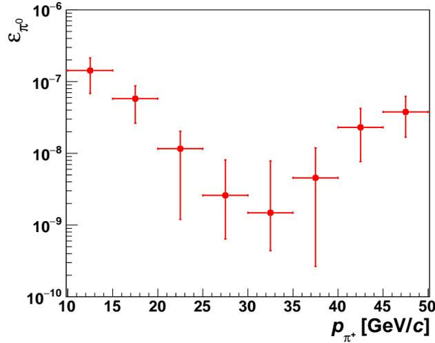
Figure 11: Expected background rejection  $\epsilon_{\pi^0}$  as a function of the charged pion momentum  $p_{\pi^+}$ .
