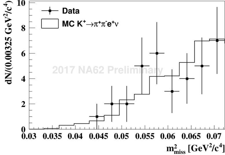
Figure 9:  $m_{miss}^2$  of a  $K^+ \rightarrow \pi^+\pi^-e^+\nu$  enriched sample of events used to validate the  $K^+ \rightarrow \pi^+\pi^-e^+\nu$  Monte Carlo simulation. Dots are data, solid histogram Monte Carlo.
