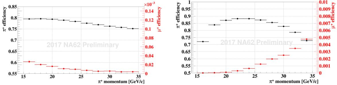
Figure 4:  $\pi^+$  and  $\mu^+$  selection efficiency after applying particle identification criteria with calorimeters (left) and RICH (right).
