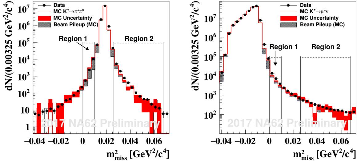
Figure 7: Distributions of the  $m^2_{miss}$  of  $K^+ \rightarrow \pi^+\pi^0$  (left) and  $K^+ \rightarrow \mu^+\nu$  (right) events used to measure the tails of  $m^2_{miss}$ . Monte Carlo prediction is also shown. The solid red bands indicate the  $1\sigma$  systematic uncertainty of the Monte Carlo. The dark shadow bands illustrate the contribution of the beam pileup to  $m^2_{miss}$  tails, as predicted from simulation.
