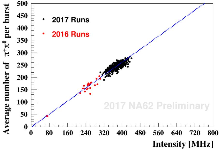
Figure 6: Average number of  $K^+ \rightarrow \pi^+\pi^0$  decays per burst selected for normalization in some of the 2016 and 2017 runs as a function of the corresponding average beam intensity. The design nominal beam intensity is 750 MHz at GTK3 (under the assumption of 3 s effective spill length).
