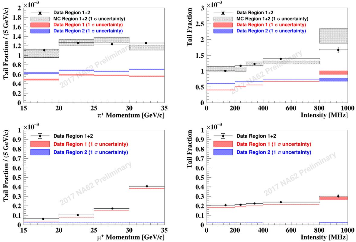
Figure 8: Fraction of  $K^+ \rightarrow \pi^+\pi^0$  (top) and  $K^+ \rightarrow \mu^+\nu$  (bottom) events entering regions 1 and 2 in bins of momentum (left) and intensity (right). Dots are data summed up in region 1 and 2. Red and blue boxes are data plotted separately for region 1 and 2, respectively. Grey shaded display the prediction from Monte Carlo simulation. The size of the boxes corresponds to  $1\sigma$  statistical uncertainty.
