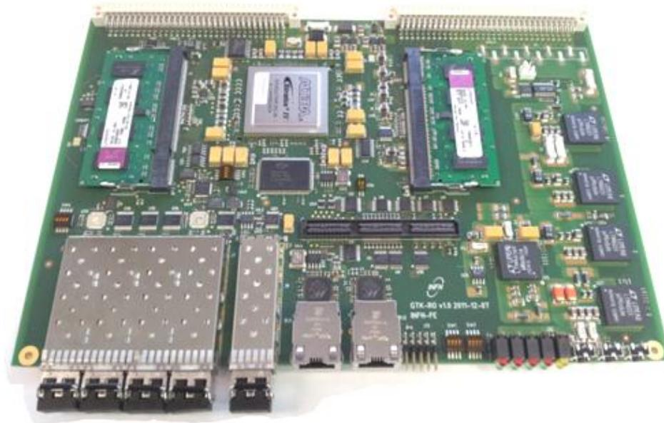
Figure 13: The prototype GTK-RO motherboard.
