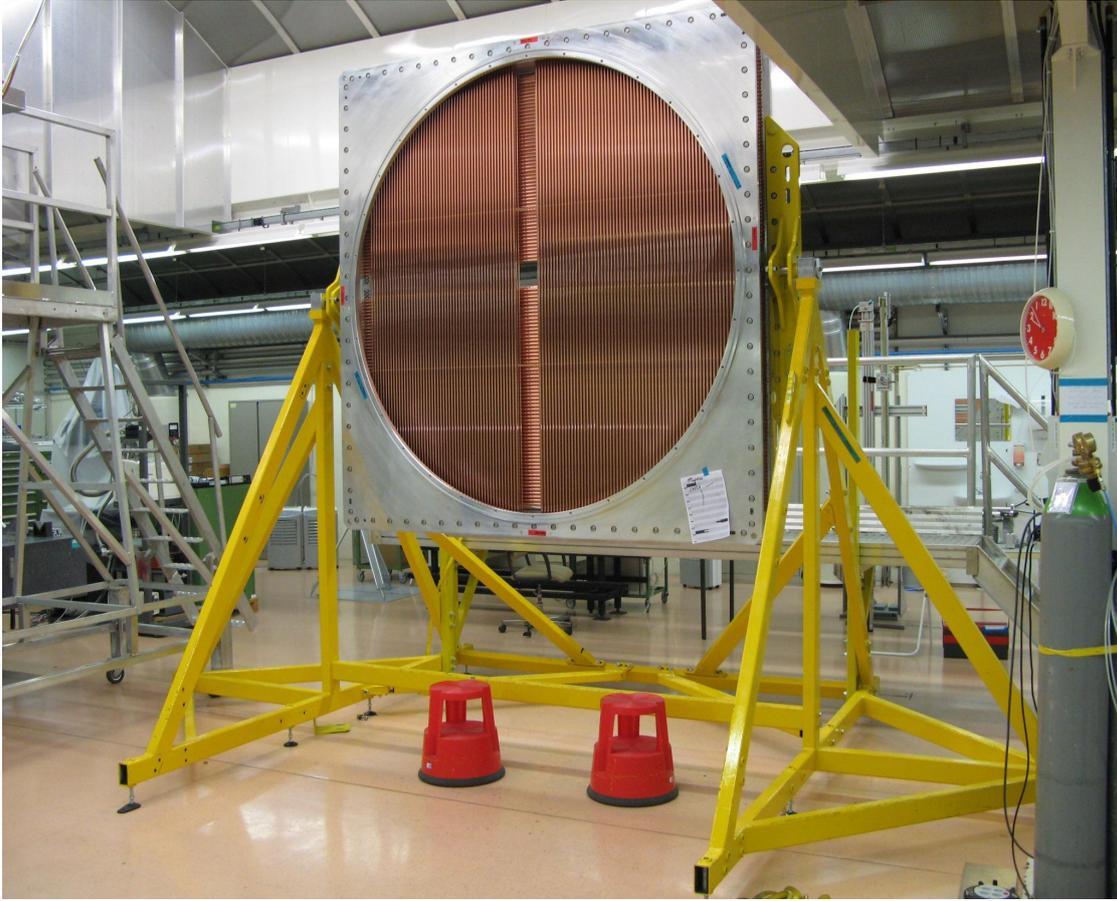
Figure 14: Completion of the straw installation after verification of straw straightness and leak tightness.
