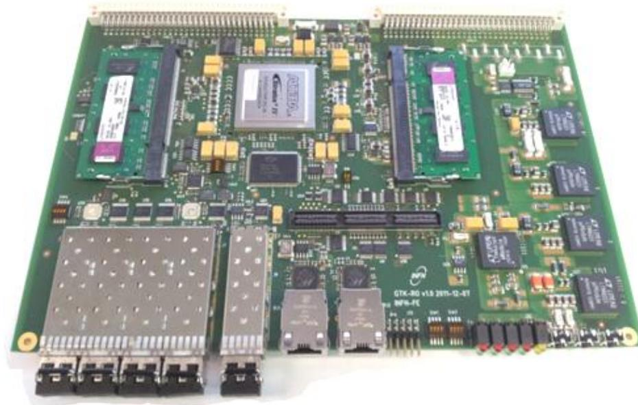
Figure 13: The prototype GTK-RO motherboard.
