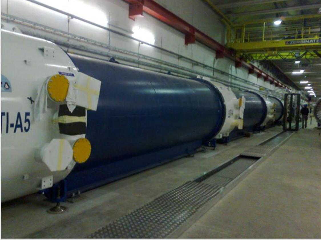
Figure 4: Installed vacuum tanks and LAV detectors in TCC8.
